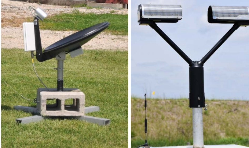
Figure 3.5: Left, the METEK MRR-2 Vertical K-band radar profiler stationed at Vierkandt Farms. Right, the Automated Parsivel Unit APU03 disdrometer deployed near XPOL-2. Photo credit: Daniel Ceynar.
